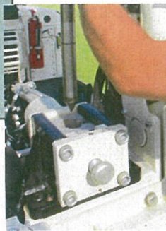
CPT Chuck for static push tooling.
